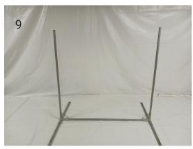
10&11. Attach elbow fittings to ends of connected poles. Tighten eye bolts to secure poles to fittings.
