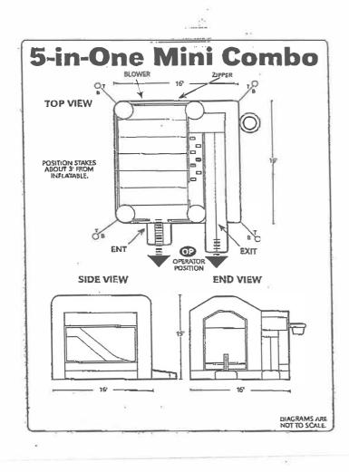
Recommended Number Maximum Number of of Number of Installers Patrons Operators 6 1 1 Total Passenger Suggested Max Weight Weight per Patron 150 lbs. 1,200 lbs. Use Whistle for Control Indoor Outdoor No. of Stakes Minimum Weight Hard-& Maximum & Minimum Container Surface Anchors Anchors\* Height Stake Length (4) 1,000 lbs. 60" (4) 40" Long (4) 600 lbs. Max. 36" Min, 75% Buried 150 lbs. 250 lbs. Per Contair Por G
