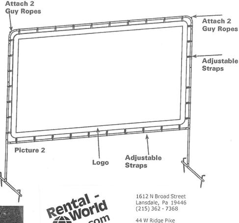
Using the supplied guy wires and stakes secure the frame to prevent it from moving around in windy conditions or tipping over.
