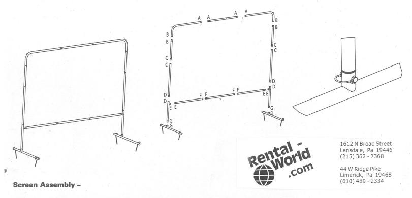
Slide the screen over the top of the frame of the screen centering the screen left to right as you go. The screen should be on the same side as the long part of the legs.
