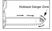
grip with thumbs and fingers encircling the chainsaw handles. A firm grip will help you reduce kickback and maintain control of the saw. Don't let go.
