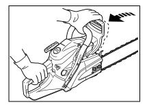
3. Hold the bar nose up, and turn the adjuster toward (+) until chain contacts underside of the bar.
