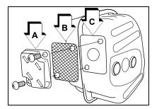
Note: When cleaning carbon deposit, be careful not to damage the catalytic element inside muffler.
