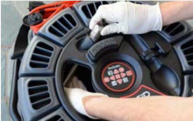
Figure 12 – Route camera head through camera access opening.
