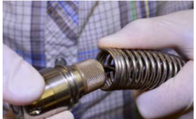
4. Rotate the camera head one turn counterclockwise and then thread it onto the spring to counteract the twisting that will occur when twisting.
