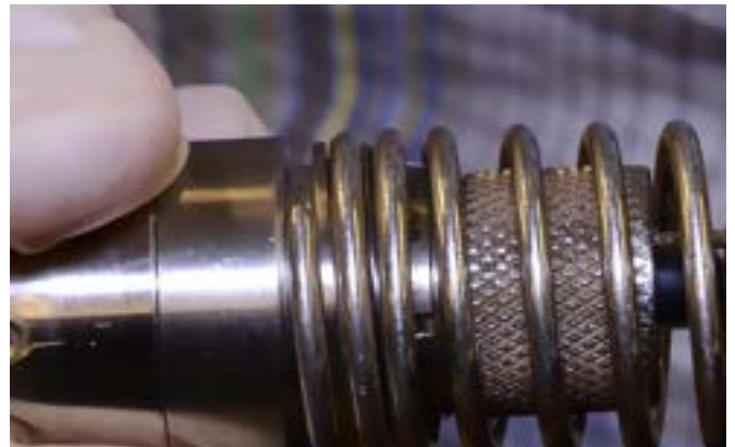
5. Thread the spring onto the camera head until the end of the spring is flush against the camera head.
