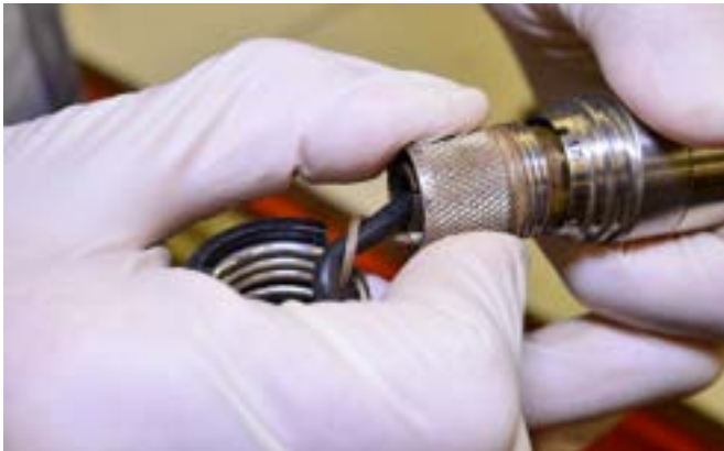
3. Hold the camera head and screw the locking sleeve back into the camera head.
