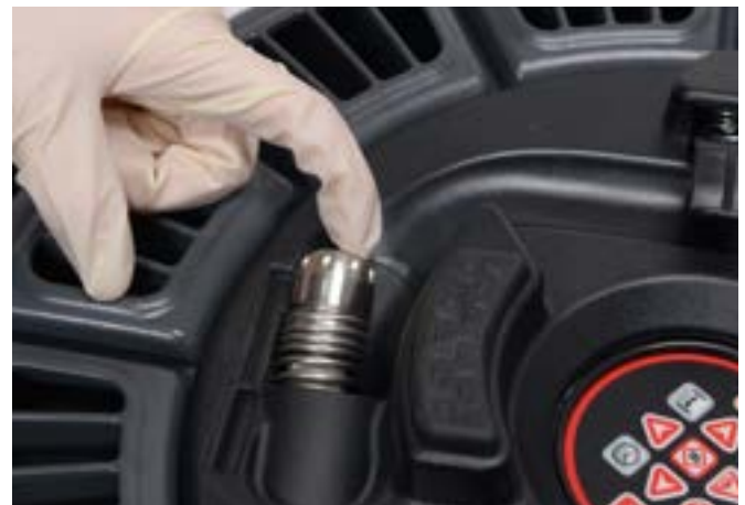
Figure 22 – Push camera head into internal drum
