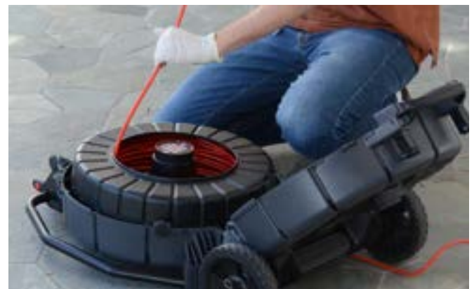
Figure 15 – Guiding the push cable into the drum
