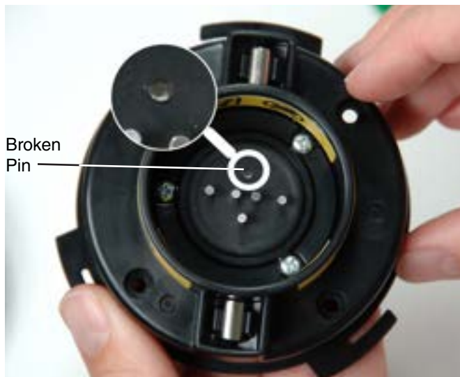
Figure 16 – Broken contact pin
