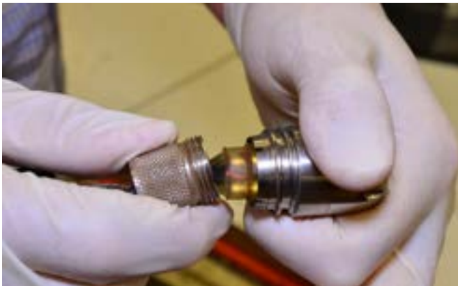
2. Slide push cable locking sleeve into camera head.
