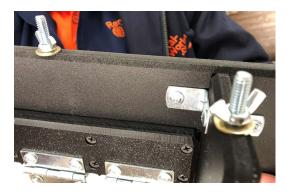
3.) Line up clown head to the holes in the base. Washers are on the front side and wing nuts are on the bottom. Tighten the wing nuts.
