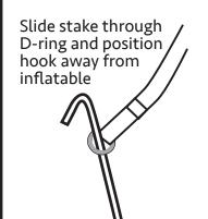
Anchor straps should be fully extended, away from unit
