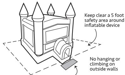
ASTM Int'l guideline calls for a 4 ft. Impact Mat at entry and exit points—center either a 4x4, 4x6 or 4x8 mat at each opening
