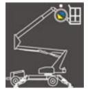
Press (push) the JIB RAISE / LOWER ( 21 ) button until the LED is lit. Pressing (squeezing) the ENABLE LEVER on the JOYSTICK, enables the function. Using the color-coded direction arrows, move the JOYSTICK slightly off center; move the JOYSTICK forward to raise the jib boom, move the JOYSTICK backwards to lower the boom.
