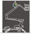
Press (push) the SECONDARY BOOM EXTEND / RETRACT (18) button until the LED is lit. Pressing (squeezing) the ENABLE LEVER on the JOYSTICK, enables the function. Using the color-coded direction arrows, move the JOYSTICK slightly off center; move the JOYSTICK backwards to extend the secondary boom, move the JOYSTICK forward to retract the secondary boom.
